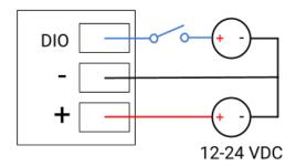
The Digital Input provides a way to locally manage SecureEdge Pro's VPN connection (ON/OFF). The wiring for proper operation of Digital Input (DI) is depicted in the image above.
