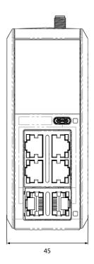
The SecureEdge Pro is designed to be cooled using natural convection. For proper cooling, you must provide a clearance of at least 35 mm above and below the device. Also, allow at least 35 mm of depth between the front of the device and the inside of the control cabinet.
