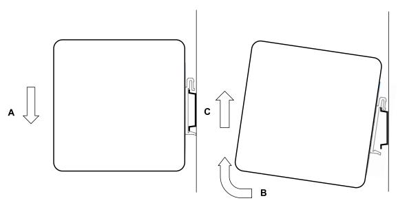
To remove the unit, (A) push the device down, (B) pull and rotate the device up and (C) lift off the rail.
